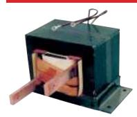
The heart of the S.W.A.T. Welder is the extended service transformer. This 10 volt transformer has an extended duty cycle because of its thermal mass (53 pounds of transformer laminate) BIGGER than any competitor. Oversized copper windings (6.5 pounds of #8 square wire on the primary, and 8 pounds of 1 inch by 3/8 inch bar on the secondary) minimize heat-build in heavyduty use.
