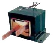
The heart of the DiGi S.W.A.T. Welder is the extended service transformer. This 10 volt transformer has an extended duty cycle because of its thermal mass (53 pounds of transformer laminate) <u>BIGGER than any competitor</u>. Oversized copper windings (6.5 pounds of #8 square wire on the primary, and 8 pounds of 1 inch by 3/8 inch bar on the secondary) minimize heat-build in heavy-duty use.
